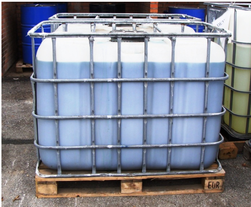
Figure B.1: example of a 600 litre reusable tank (intermediate bulk container) used for the transport of liquid detergents to retail establishments when the product is to be distributed loose through self-dispensing systems. The image was taken during a survey of the manufacturing and packaging plant of a medium-sized company located in central Italy.
