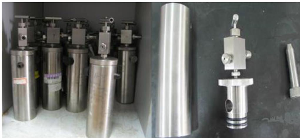
FIGURE 5.1 High pressure metallic vessels used for batch incubations at 100 bar.
