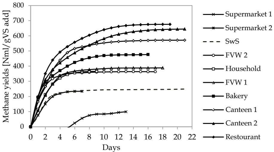
Figure 2.3 Cumulative methane yields curves of SS-OFMSW and SwS.
