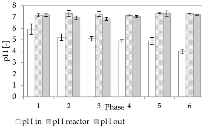
**Figure 3.21** pH values during the experimental phases.
