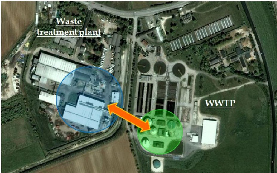
**Figure 5.1** WWTP and waste treatment plant aerial photo with in blue circle the OFMSW collection building and the composting plant, in the green circle the AD unit inside WWTP.
