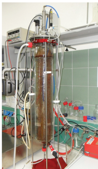
FIG. 6.4 Anammox biofilm gas-lift suspension reactor.
