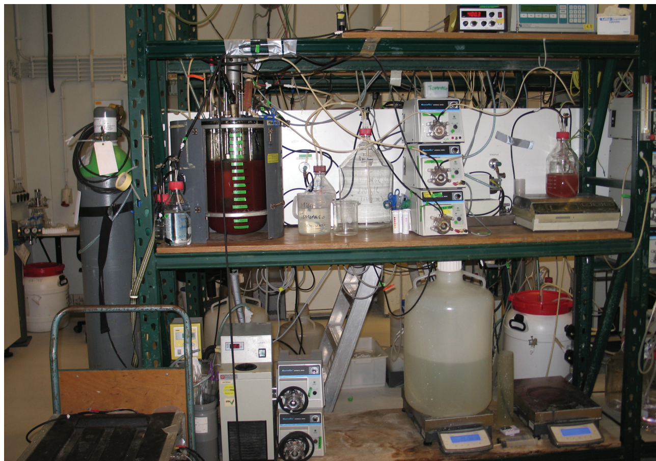
FIG. 3.2 Photograph of the set-up of the membrane bioreactor (MBR) for enrichment of anammox bacteria as free cells.
