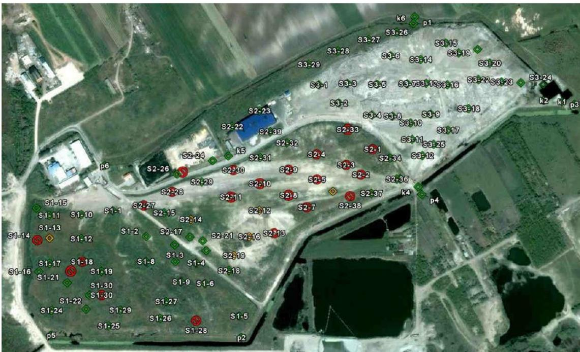
Figure 14: Novi Sad landfill gas wells layout (from Vujic et al., 2012)
