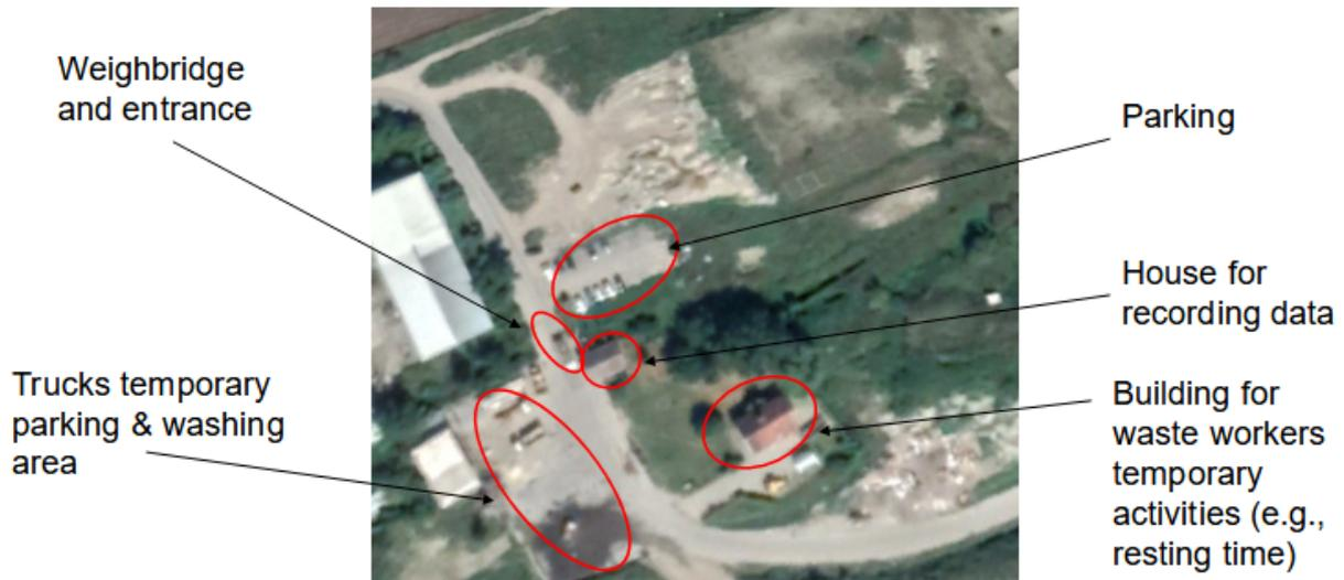
Figure 12: Elements characterizing the landfill entrance area (from Google Earth - Modified)
