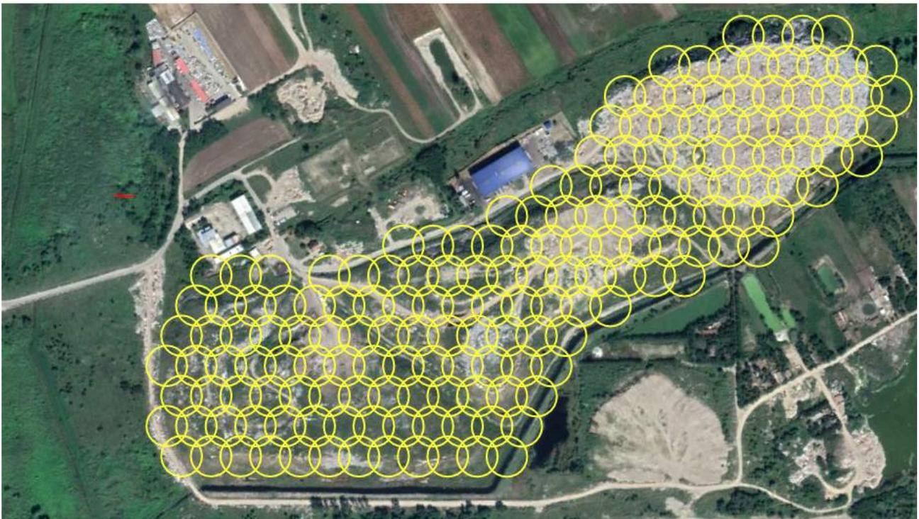
*Figure 28: Proposed distribution of wells for biogas extraction, with a ROI of 25 m*
